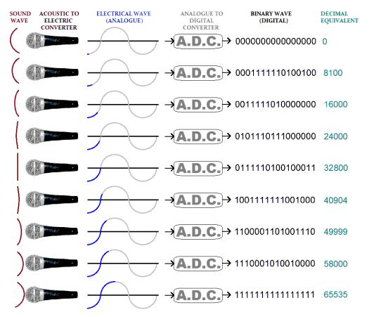
Digital recording involves converting the incoming Analogue signal from the microphone into Digital numbers using an Analog-to-Digital converter. Once in the digital domain modern software offers us tremendous opportunities to manipulate the sound without any noticeable loss of quality.
